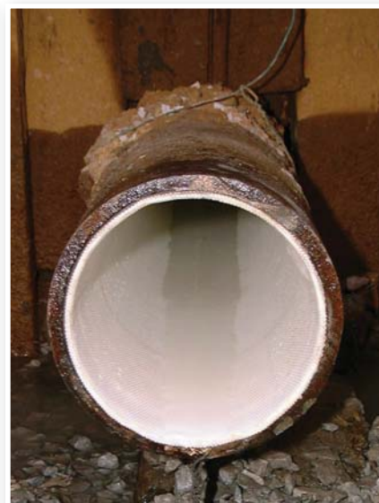
Section of pipe with liner installed and cured.
